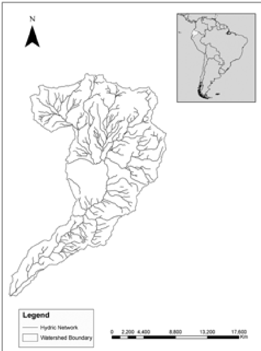
Figure 20: Drainage network of the El Angel Watershed
